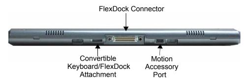
*FlexDock Connector.* There is a FlexDock connector at the bottom edge of the Tablet Client. This connector mates with the corresponding connector on the FlexDock for the LE Series to provide the required signal connections when the Tablet Client is "docked." Refer to the Installation Guide provided with the FlexDock for the LE series unit for more information.
